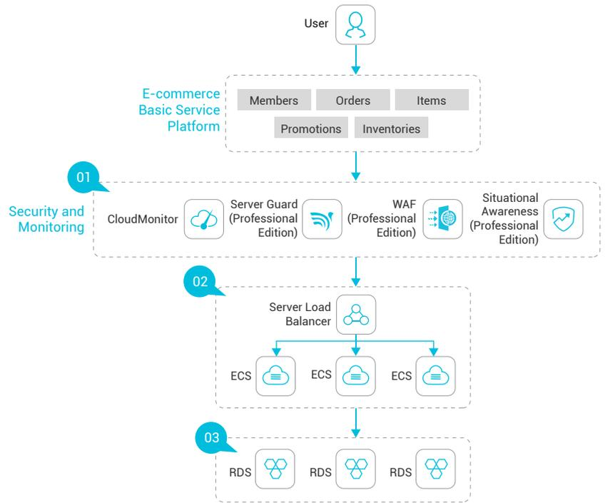
This architecture diagram demonstrates a typical cloud solution for a small scale e-commerce setup.
