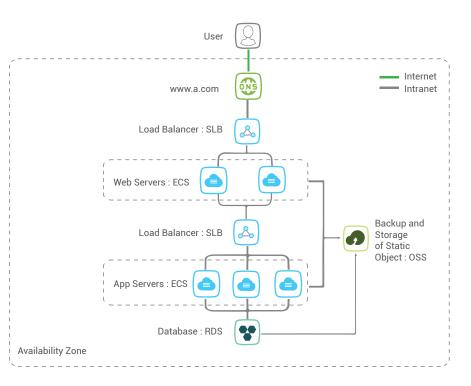
This architecture diagram illustrates a typical web application hosting architecture using Alibaba Cloud services:
