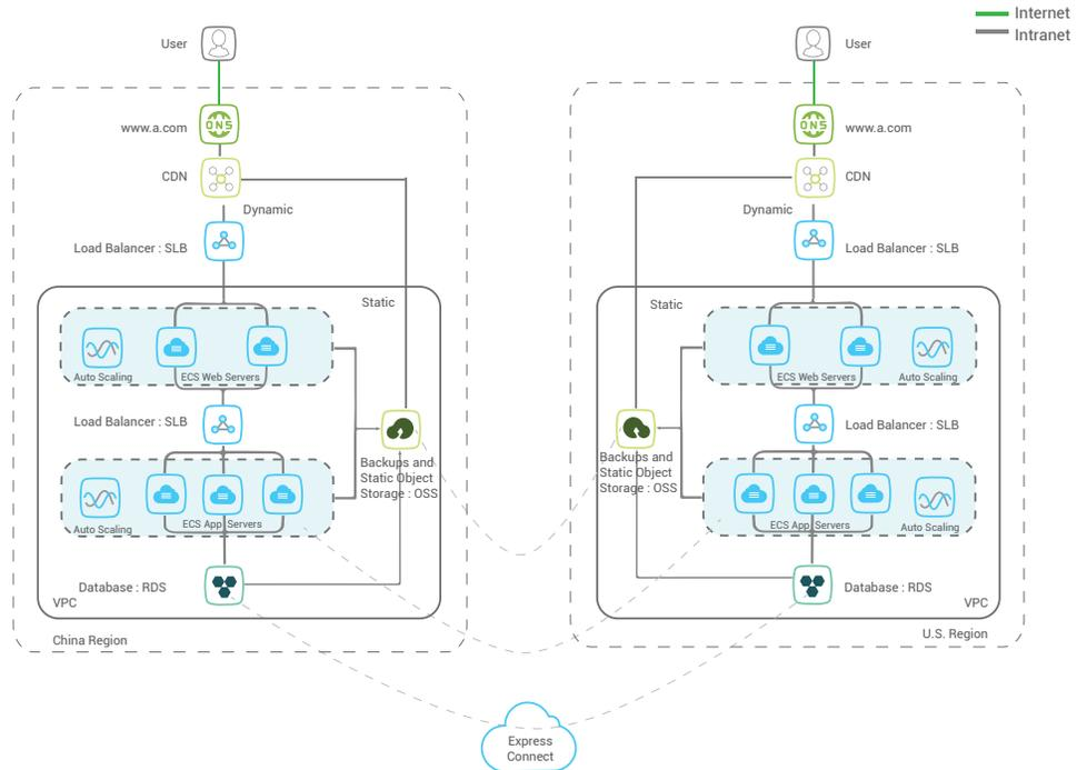
1. User request is received and served by the nearest DNS server, and automatically routed to the CDN for accelerated content delivery.
